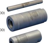
ExpanTek® Tube Expansion Tools offer fast, snap-on coupling and positive sealing for high-pressure expansion of tubes and pipes. The Hydro Ball Expansion Tool propels a chrome ball the length of the tube. Systems supply pressurized water to tool for rapid tube expansion in 2 to 3 seconds. Equipment engineered to customer application requirements.
