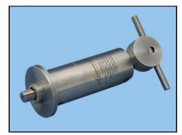
The propriety collet design is the key feature of the Model 350 Tool. When the tool is engaged in the threaded area of the test piece, it does not mark or deform the threaded surface. This tool provides positive sealing on the end face of the internally-threaded port. Pressure compensation in the tool increases the sealing force, and ensures the collets remain engaged with the component
