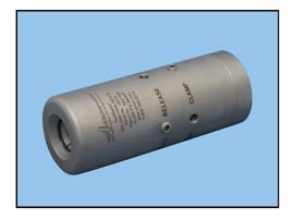
The pressure compensated design of the Model 500 Tool places the tube or pipe in tension, using internal pressure to grip and seal on the tube OD. This design eliminates tube clamping devices along the tube length. One body size will accommodate multiple wall thicknesses, while maintaining high fill rates.
