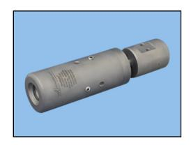
The pressure compensated design of the Model 525 Tool places the tube or pipe in tension, using internal pressure to grip and seal on the tube OD. This design eliminates tube clamping devices along the length of the tube. One body size will accommodate multiple wall thicknesses, while maintaining high fill rates.
