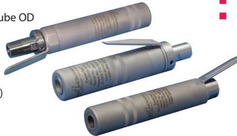
*ExpanTek<sup>®</sup> Tube Expansion Tools offer fast, snap-on coupling and positive sealing for high-pressure expansion of tubes and pipes. The Hydro Ball Expansion Tool propels a chrome ball the length of the tube. Systems supply pressurized water to tool for rapid tube expansion in 2 to 3 seconds. Equipment engineered to customer application requirements.*
